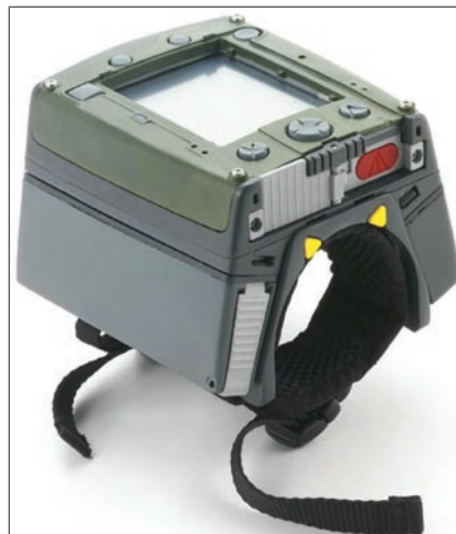
Figure 4 displays the latest version of the Zypad, the WR1100, designed to meet strict military requirements.
