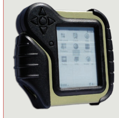
FIGURE 2: The SFPDA, designed for longer missions in the field, has a typical power consumption well under 1 W, including device display and a standard peripheral set.
