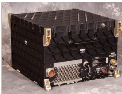
FIGURE 2: The ASIP's enclosure, a configuration of the direct spray cooled MPE, is designed to environmentally isolate sensitive electronics and provide necessary thermal management.
